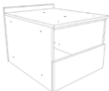
MB107 - Open Void with Half Height False Drawer Front 637(L) x 800/950(W) x 519(H)
