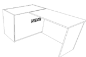
Peninsular Teachers Desk Unit Width Varies x 730(H) x up to 590(D) TW109 - 1000mm wide TW110 - 1040mm wide for use with Tray Unit TW111 - 1078mm wide for use with Tray Unit with Doors
